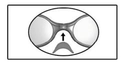
Carefully insert the nose into the frame, by hand or using a pair of suitable pliers.
